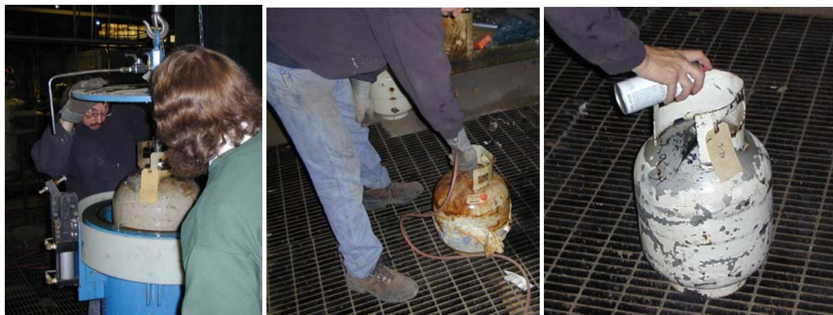
Figure A-8. Removal of the cylinder from the jacket, drying of the fracture surface with air and painting the fracture surfaces with clear acrylic paint to preserve their appearance.
