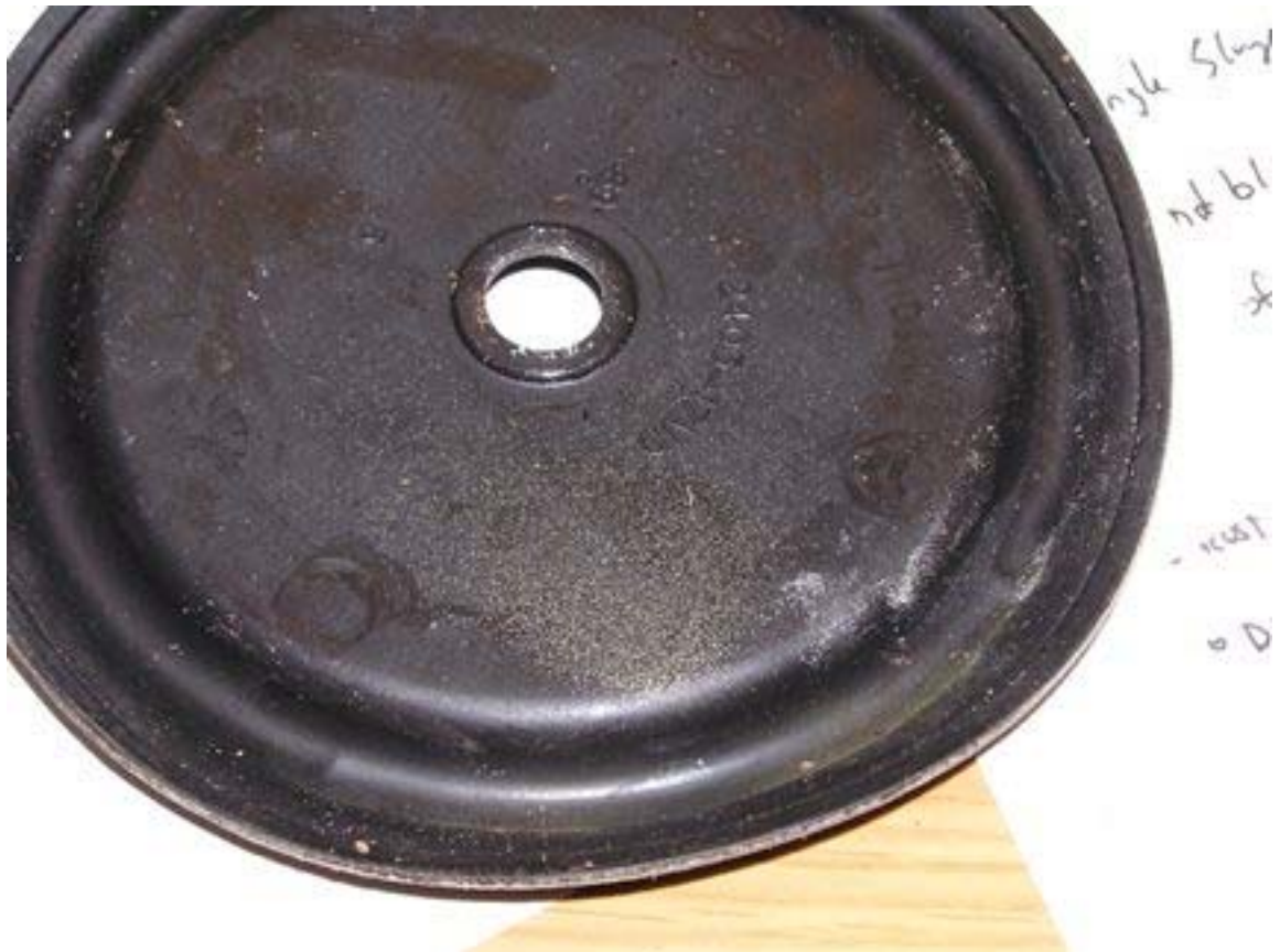
Figure 6: Bottom Side of Diaphragm (Regulator #353)
