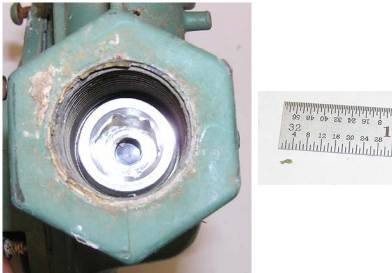
Figure 3: Debris Found on Inlet of Regulator #42
