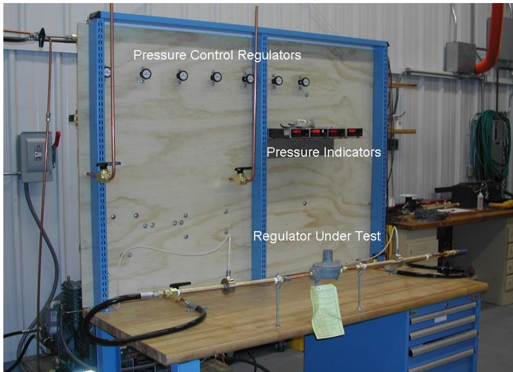
Figure 16. Regulator test stand — front view.
