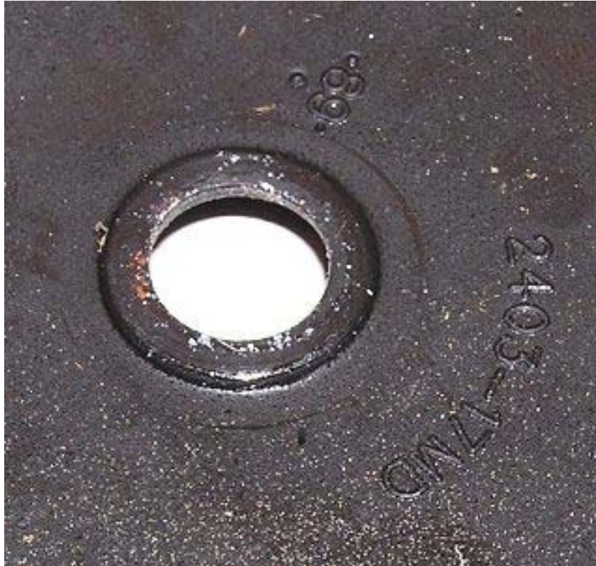
Figure 7: Debris on Sealing Surface Between Diaphragm and PRD Stem
