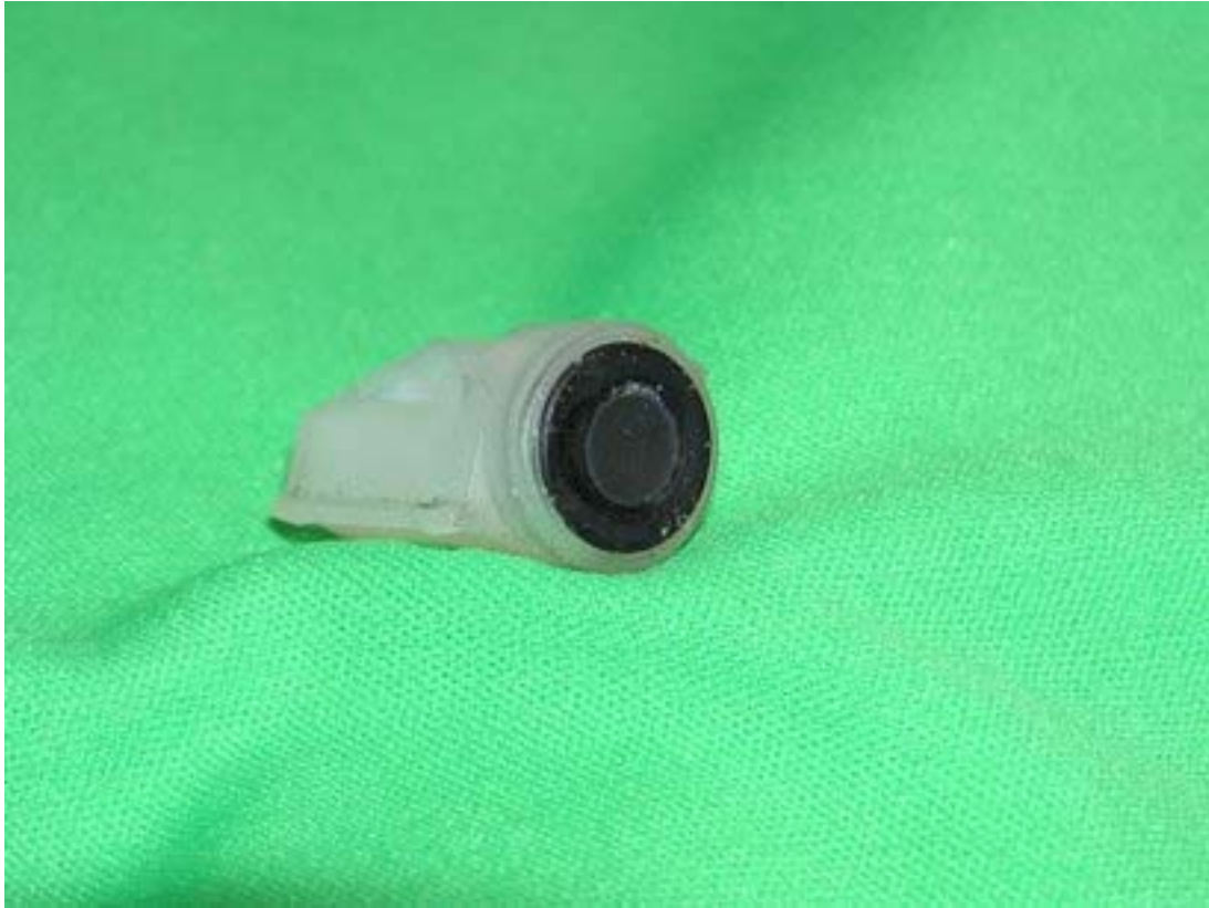
Figure 6: Seat Disc from Control Linkage (Regulator #571)
