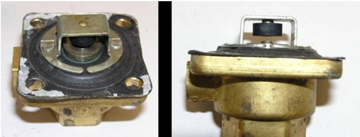
Figure 7: First-Stage Portion of Regulator #490
