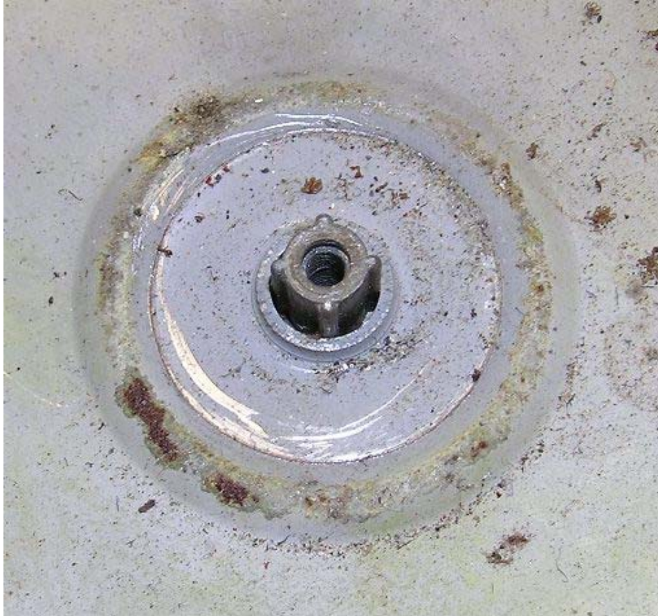
Figure 4: Scratches on Regulator #361 Diaphragm Plate
