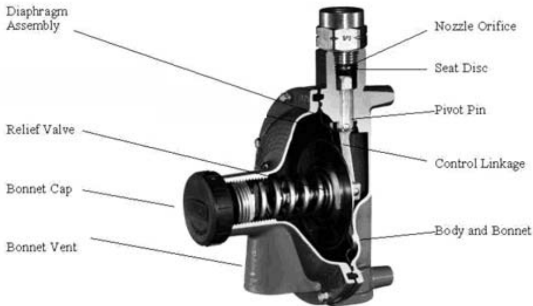
Figure 1. Components of a typical regulator. 1
