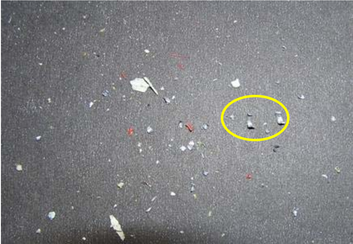
Figure 3: Particles and Shavings (circled) Found inside Bottom of Regulator #571
