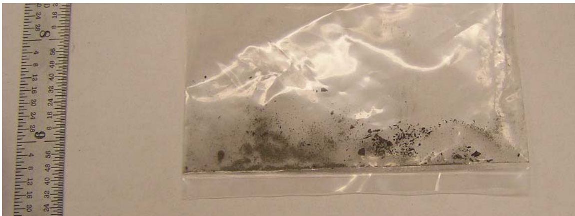
Figure 7: Dirt and Debris Removed Between Nozzle Orifice and Seat Disc
