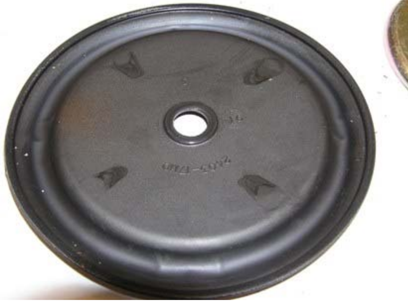
Figure 6: Bottom of Second-Stage Diaphragm (Regulator #13)
