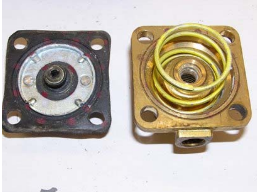
Figure 8: Inlet Side of First-Stage Portion of Regulator #490
