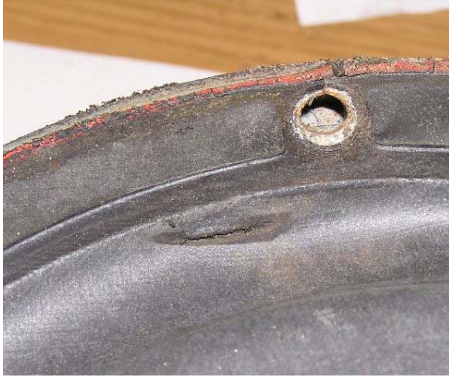
Figure 5: Cut on Bottom of Regulator #361 Diaphragm
