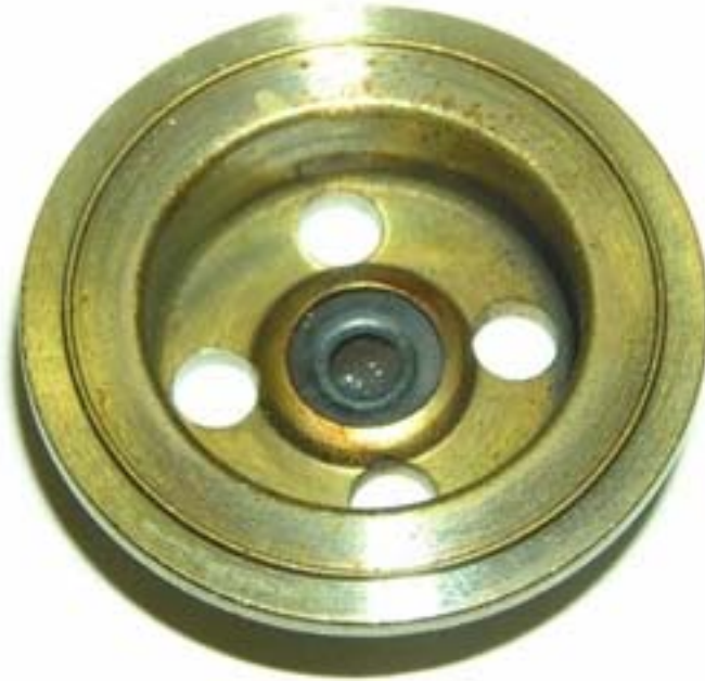
Figure 10: First-Stage Plate (Regulator #13)
