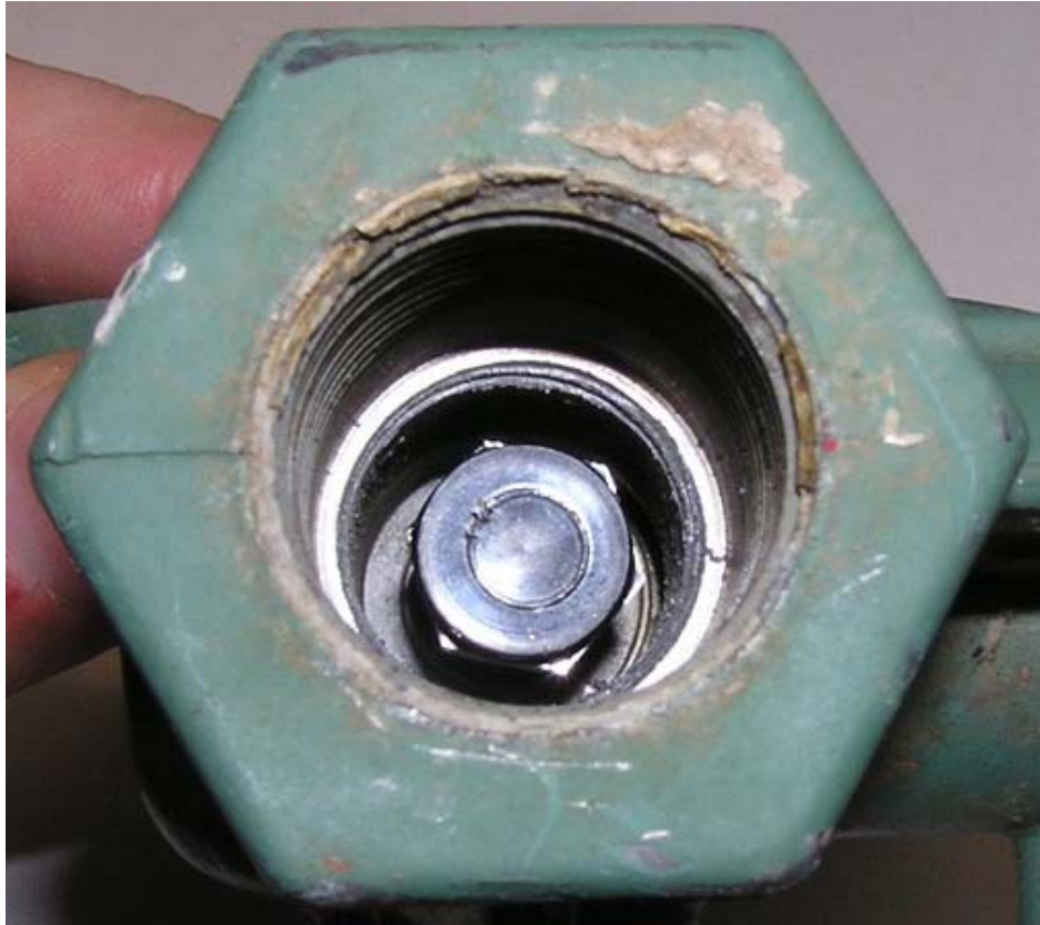
Figure 6: Damage to Inlet Seat Disc of Regulator #42
