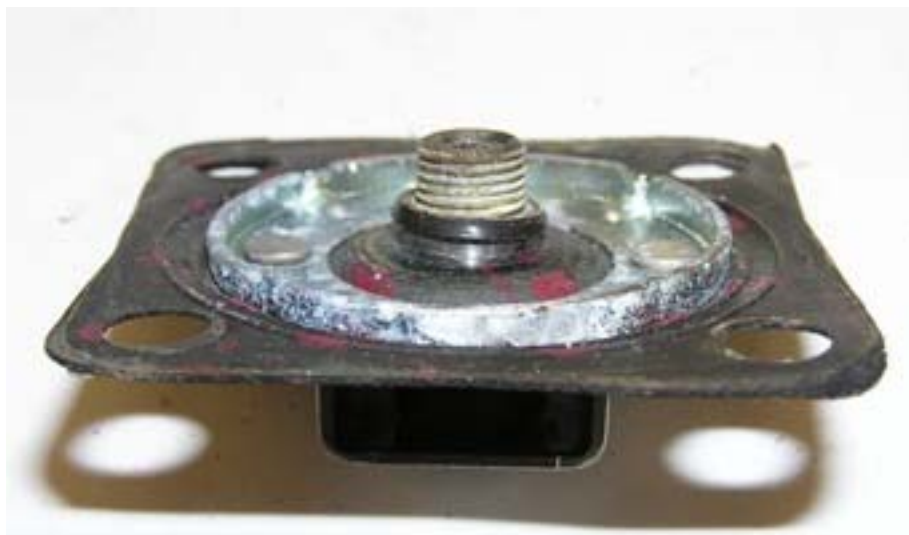
Figure 9: First-Stage Diphragm (Regulator #490)
