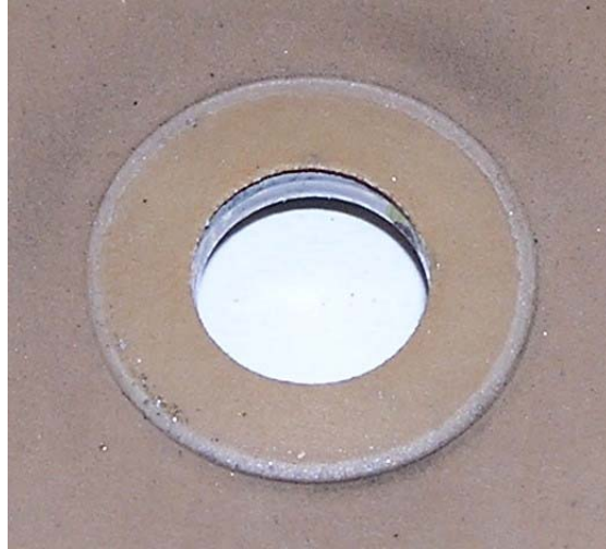
Figure 5: PRD Seal on Bottom of Regulator #383 Diaphragm
