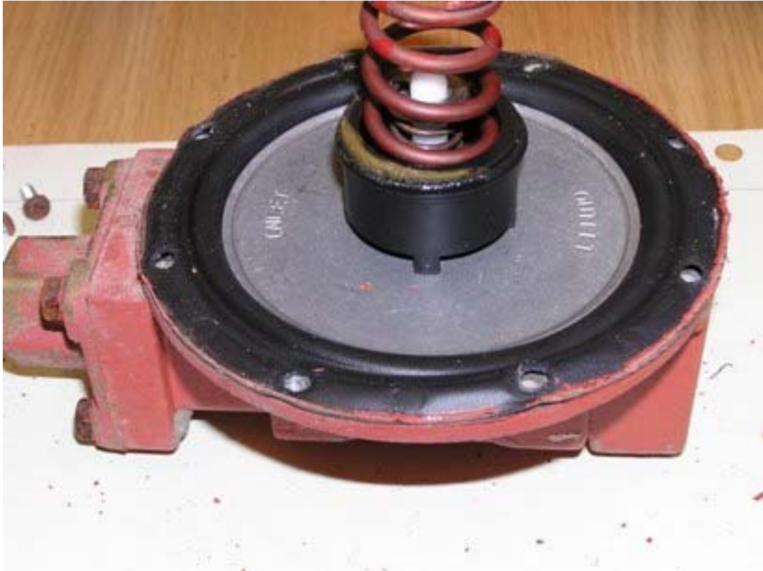
Figure 2: Regulator #571 with Top of Body Removed
