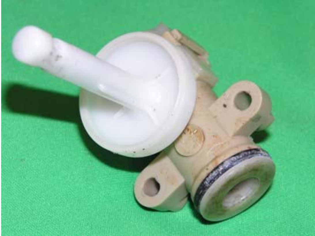
Figure 5: Control Linkage Assembly (Regulator #571)
