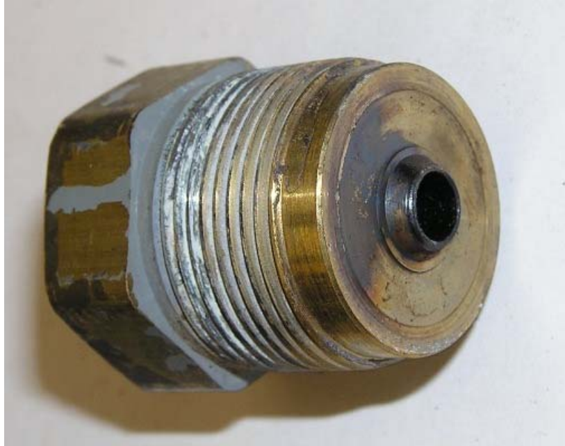
Figure 8: Nozzle Orifice of Regulator #383
