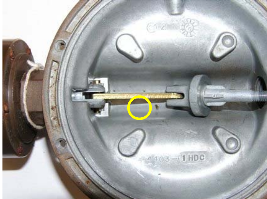
Figure 7: Bottom Body of Second-Stage (Regulator #13)
