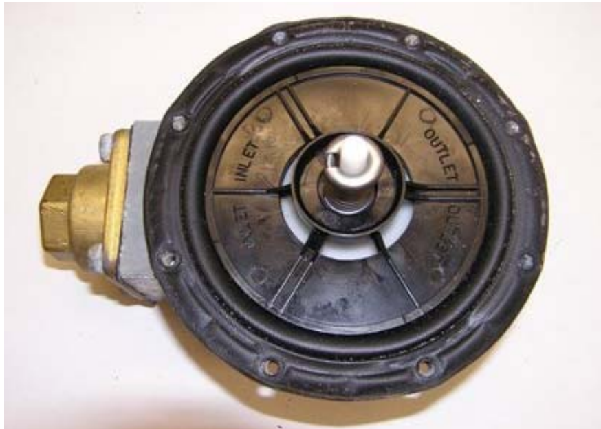
Figure 3: Top Half of Second-Stage (Regulator #490)
