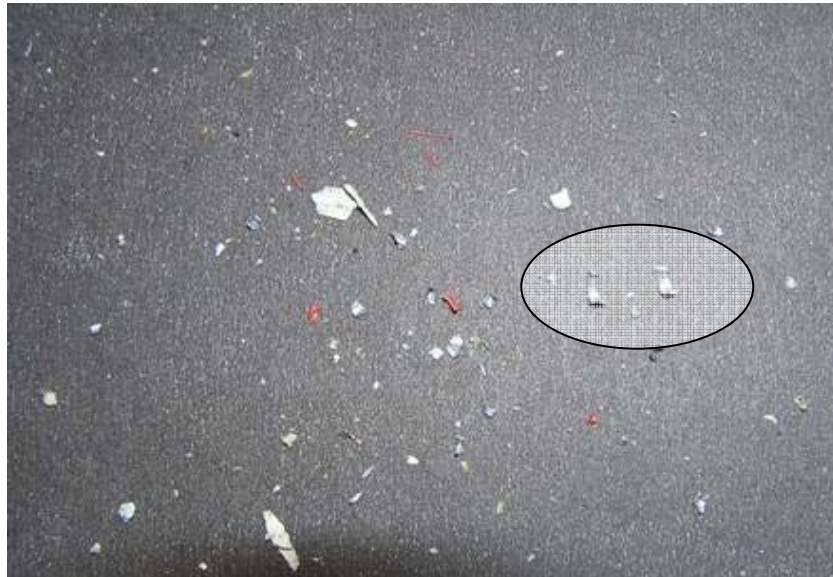
Figure 77. Regulator 571 — machining turnings found inside regulator.
